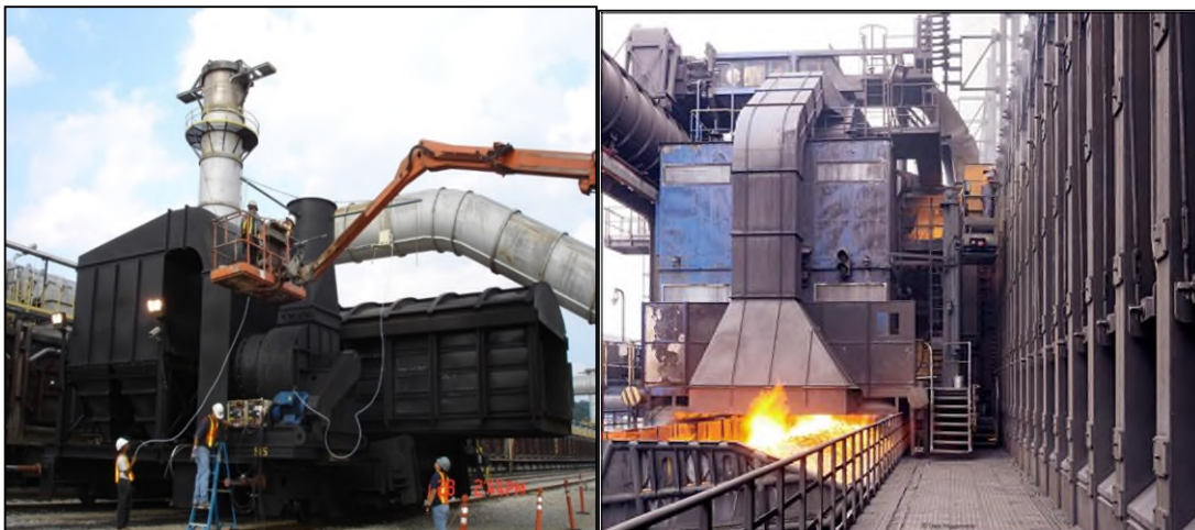
Figure 6. Nonrecovery Coke Plant Flat Push Hot Car during Sampling (left) and Byproduct Coke Plant Pushing Operations (right)
