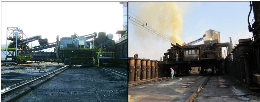
Figure 5. Nonrecovery Plant PCM Charging Operations (left) and Byproduct Plant Larry Car Charging Operations (and Coke Oven Gas Removal) (right)
